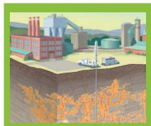
In fractured rock with primary porosity of as little as 1%, the vast majority of the contaminant mass may be present in the rock matrix rather than the fractures.
